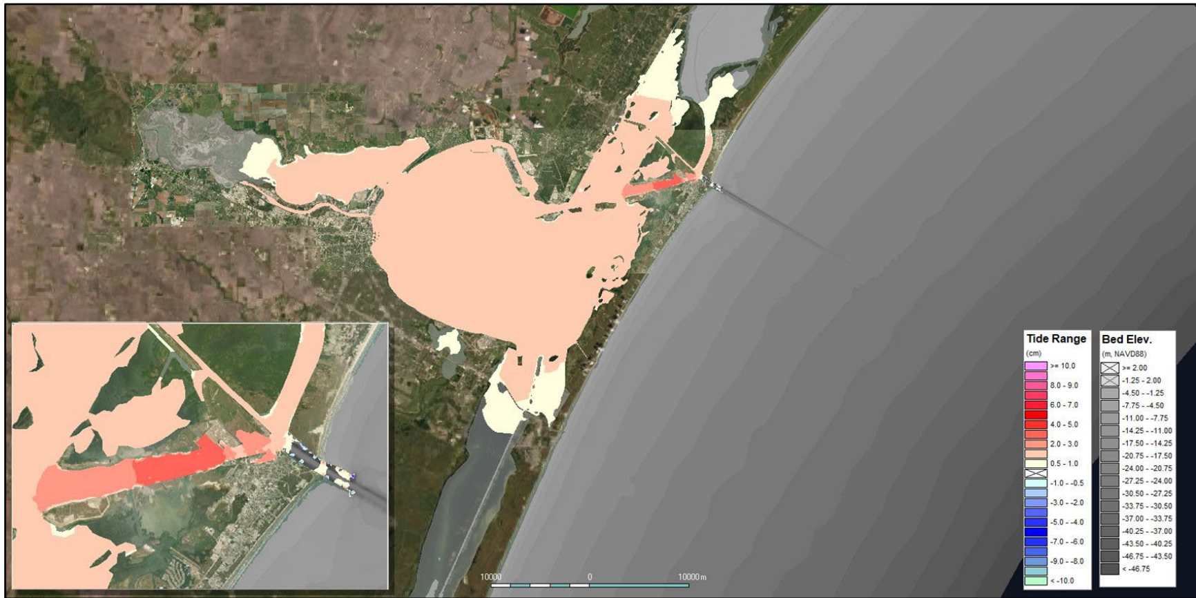
Figure 4-1. Mean Tide Range Change Caused by the Applicant's Preferred Alternative Compared to the No-Action Alternative Under Long-term Modeling
